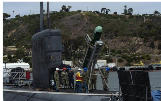
Sailors load a Mark 48 advanced capability torpedo onto the Los Angeles-class fast-attack submarine Scranton on June 24, 2021. (MCC Josue L. Escobosa/U.S. Navy)
