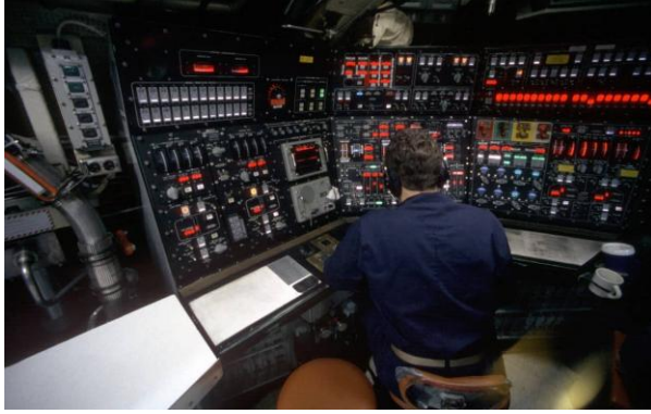
A sailor mans the main console of the ship's Ballast Control Panel on board the nuclear-powered ballistic missile submarine USS Pennsylvania (SSBN-735), USN
