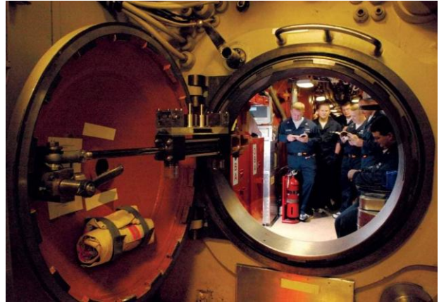
The watertight hatch that separates the rest of the boat from 'Sherwood Forest.', USN
