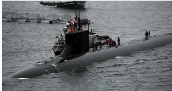
USS Connecticut has no fins attached to its vertical sail. A visual scan of Puget Sound Naval Shipyard in Bremerton, Washington, in early 2023 reveals submarines with sailfins parked or in various states of repair. SSN 22's sail has a distinctive shape and will not cast sailfin shadows. US Navy photo.
