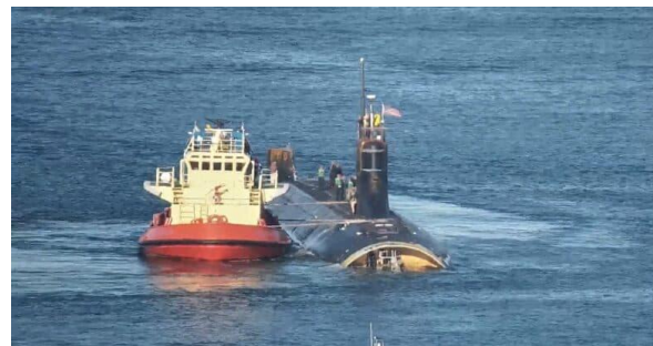
USS Connecticut (SSN 22) gets assist from a tug as it leaves San Diego harbor on December 15, 2021. Note the sheared off bow and the lack of a sonar dome. San Diego WebCam photo via USNI News
