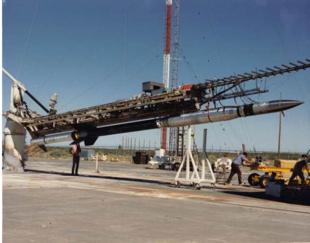
The large tilting launch rails used for Aerobee rockets at LC-35. These rockets could travel dozens of miles into the upper reaches of Earth's atmosphere. , UC Boulder
