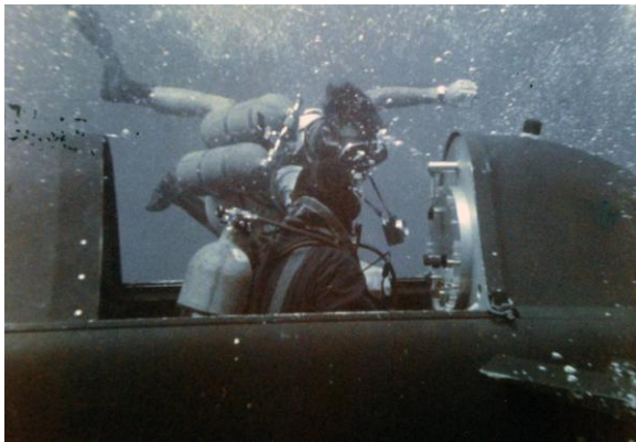
Support divers from USS Grayback ready an SDV for launch operations at a depth of 35 feet. The vehicle was manned by personnel from Underwater Demolition Team 12., National Archives
