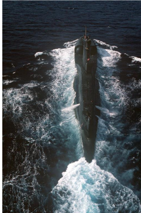
High-angle stern view of the USS Grayback underway. You can see two of the "sharkfin" sonar domes associated with the PUFFS system on the hull., National Archives
