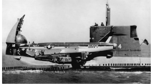
An SSM-N-9 Regulus II missile is maneuvered aboard the USS Grayback , U.S. Navy
